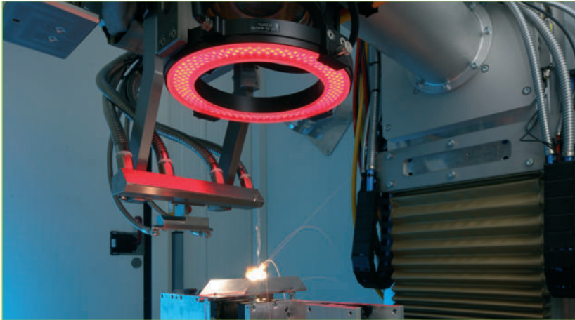
Fig. 5: Experimental cell for laser welding in order to investigate laser-based processes for joining copper materials ■
